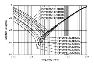
Common Mode Insertion Loss (Typ.)
