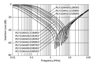
Differential Mode Insertion Loss (Typ.)
