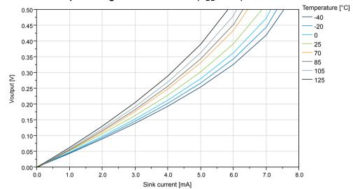
Figure 35-21. IO Pin Output Voltage vs. Sink Current (V<sub>DD</sub>=1.8V)
