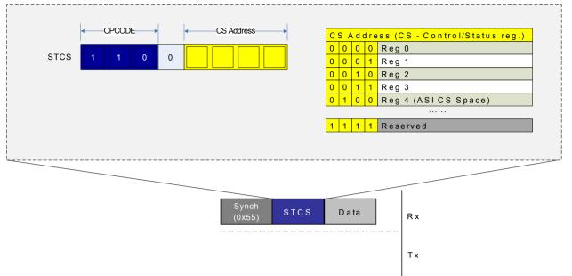
Figure 33-14 shows the data frame transmitted after the SYNCH and instruction frames. Note that there is no response generated from the STCS instruction, as is the case for ST and STS.
