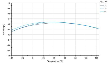
Figure 35-34. Internal 2.5V Reference vs. Temperature
