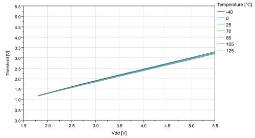
Figure 35-20. IO Pin Input Threshold Voltage vs.  $V_{\text{DD}}\left(V_{\text{IL}}\right)$
