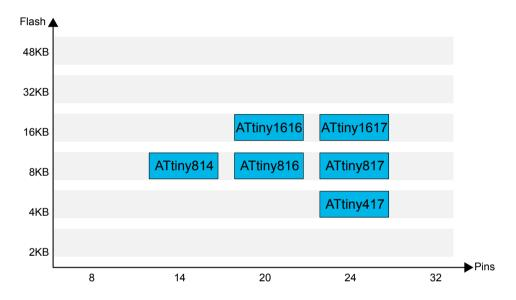
The fully compatible variants of the ATtiny devices, that is the vertical migration option in Figure 1-1, come with both smaller and larger Flash memories.
