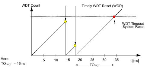
**Note:** Normal mode is enabled as long as the WINDOW bit field in the Control A register (WDT.CTRLA) is 0x0.
