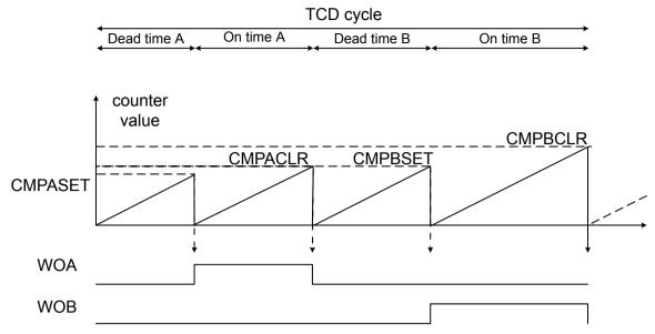
There are no restrictions on the compare values compared to each others. **Note:** In Four Ramp Mode it is not possible to get overlapping outputs.
