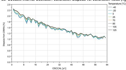
Figure 35-56. OSC20M Internal Oscillator: Calibration Stepsize vs. Calibration Value (V<sub>DD</sub>=3V)
