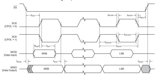
Table 34-14. USART in SPI Mode - Timing Characteristics
