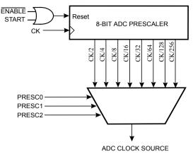
By default, the successive approximation circuitry requires an input clock frequency between 50kHz and 2MHz to get maximum resolution. If a lower resolution than 10 bits is selected, the input clock frequency to the ADC can be higher than 2MHz to get a higher sample rate.
