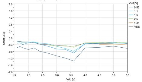
Figure 35-51. Offset Error vs. V<sub>ref</sub> (V<sub>DD</sub>=5.0V, 115ksps)
