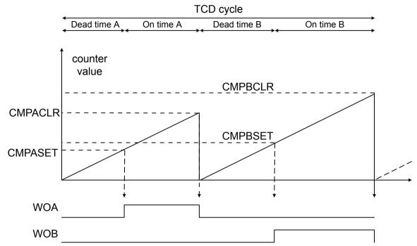
In the figure above, CMPASET < CMPACLR and CMPBSET < CMPBCLR. This causes the outputs to go high. There are no restrictions on the CMPASET/CLR compared to the CMPBSET/CLR values. **Note:** In two ramp mode it is not possible to get overlapping outputs.
