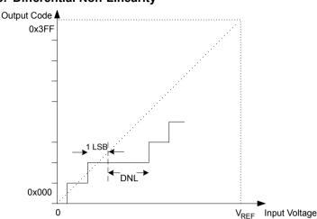
Quantization ErrorDue to the quantization of the input voltage into a finite number of codes, a range<br/>of input voltages (1 LSB wide) will code to the same value. Always ±0.5 LSB.AbsoluteThe maximum deviation of an actual (unadjusted) transition compared to an ideal<br/>transition for any code. This is the compound effect of all aforementioned errors.<br/>Ideal value: ±0.5 LSB.
