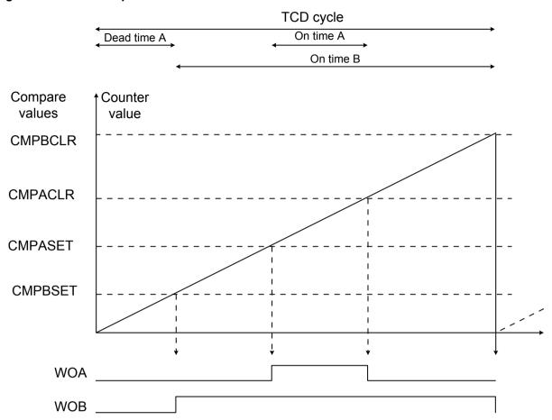
Figure 22-3. One Ramp Mode with CMPBSET < CMPASET
