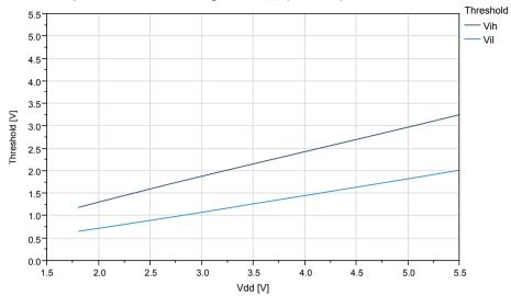
Figure 35-19. IO Pin Input Threshold Voltage vs.  $V_{DD}$  (V<sub>IH</sub>)
