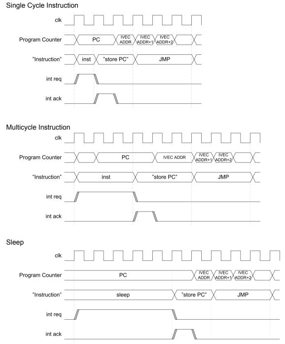
If an interrupt occurs when the device is in sleep mode, the interrupt execution response time is increased by five clock cycles. In addition, the response time is increased by the start-up time from the selected sleep mode.
