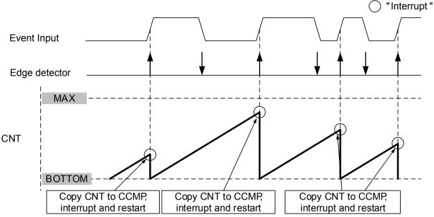
**Note:** The event pulse needs to be longer than one system clock cycle in order to guarantee edge detection.
