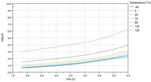
Figure 35-15. Standby Mode Supply Current vs. V<sub>DD</sub> (Sampled BOD running at 125Hz)
