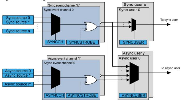
Figure 14-2. Example of Event Source, Generator, User, and Action Event Generator
