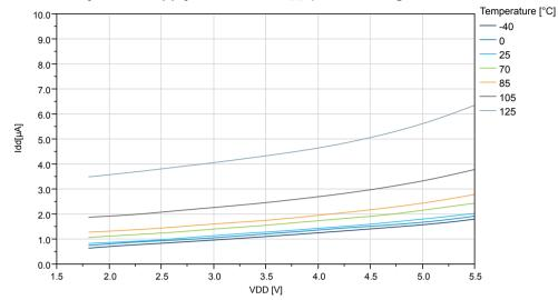
Figure 35-13. Standby Mode Supply Current vs. V<sub>DD</sub> (RTC running with external 32KHz osc.)
