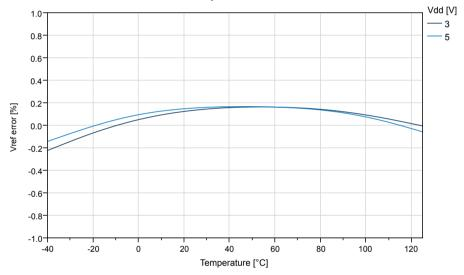
Figure 35-35. Internal 4.34V Reference vs. Temperature
