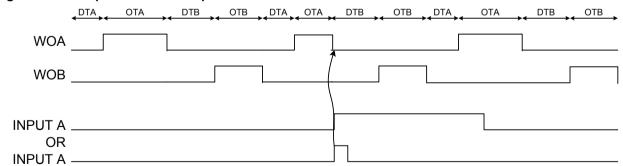
If Input mode 8 is used on input B and an positive input event occurs while in On time B, the TCD counter jumps to Dead time A.
