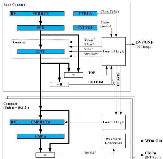
Figure 20-2. Timer/Counter Block Diagram
