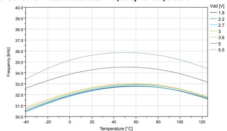
Figure 35-60. OSCULP32K Internal Oscillator Frequency vs. Temperature
