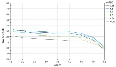
Figure 35-47. Gain Error vs. V<sub>ref</sub> (V<sub>DD</sub>=5.0V, 115ksps)
