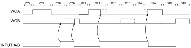
Input Mode 5: Stop all Outputs, Execute Dead Time while Fault Active
