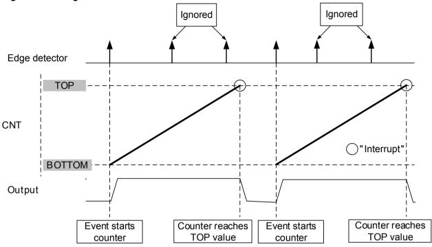
**Note:** If the ASYNC bit in TCB.CTRLB is '0', the event pulse needs to be longer than one system clock cycle in order to guarantee edge detection.
