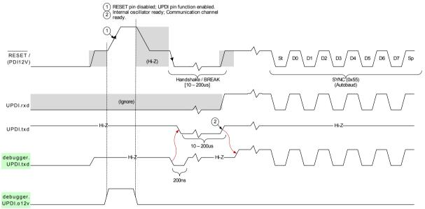
When enabled by 12V, only a POR will disable the UPDI configuration on the RESET pin, and restore the default setting. If issuing a UPDI disable command through the UPDIDIS bit in UPDI.CTRLB, the UPDI will be reset and the clock request will be canceled, but the RESET pin will remain in UPDI configuration.
