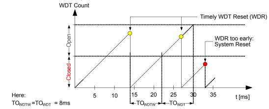
**Note:** The window mode is enabled by writing a non-zero value to the WINDOW bit field in the Control A register (WDT.CTRLA), and disabled by writing WINDOW=0x0.
