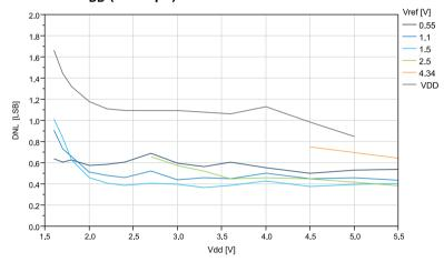
Figure 35-45. DNL vs. V<sub>ref</sub> (V<sub>DD</sub>=5.0V, 115ksps)
