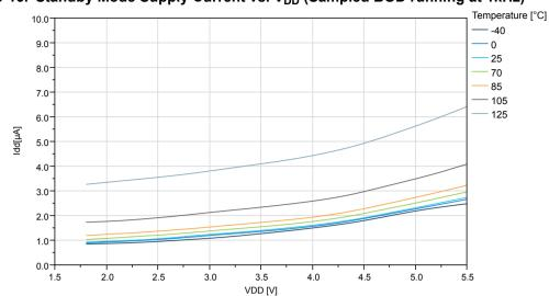
Figure 35-16. Standby Mode Supply Current vs. V<sub>DD</sub> (Sampled BOD running at 1kHz)
