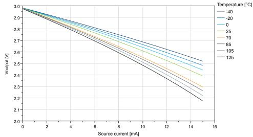
Figure 35-26. IO Pin Output Voltage vs. Source Current (V<sub>DD</sub>=3.0V)
