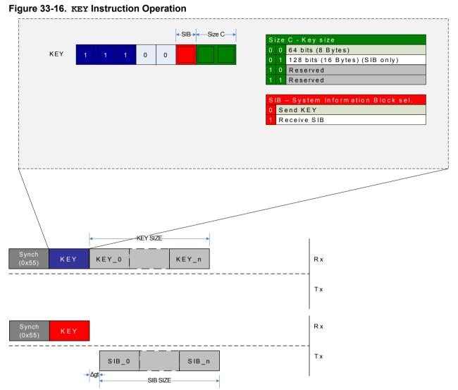
The Figure above shows the transmission of a KEY, and the reception of a SIB. In both cases, the  $SIZE_C$  field in the opcode determines the number of frames to be sent or received. Note that there is no response after sending a KEY to the UPDI. When requesting the SIB, data will be transmitted from the UPDI according to the current Guard Time setting.
