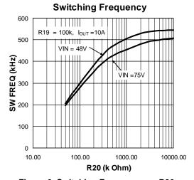
Figure 6. Switching Frequency vs. R20
