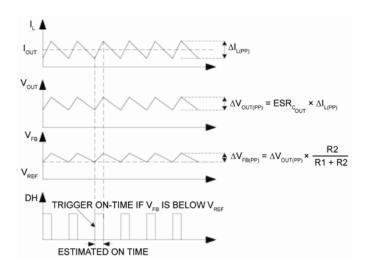
Figure 2. MIC2103/04 Control Loop Timing
