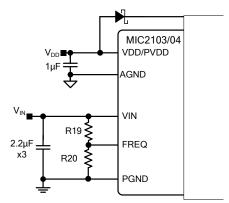
Figure 5. Switching Frequency Adjustment
