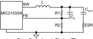
Figure 8b. Inadequate Ripple at FB
