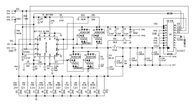
Figure 9. Schematic of MIC2103/04 Evaluation Board (J1, J9, J12, R14, and R21 are for testing purposes)
