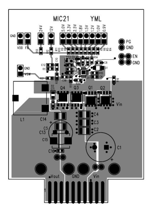
Figure 10. MIC2103/04 Evaluation Board Top Layer
