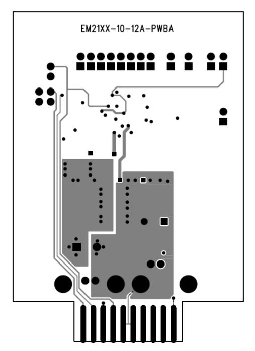
Figure 13. MIC2103/04 Evaluation Board Bottom Layer
