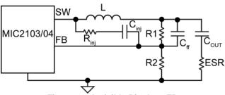
Figure 8c. Invisible Ripple at FB
