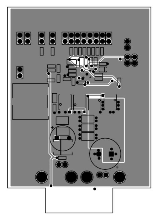
Figure 12. MIC2103/04 Evaluation Board Mid-Layer 2
