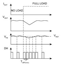
Figure 3a. MIC2103/04 Load Transient Response
