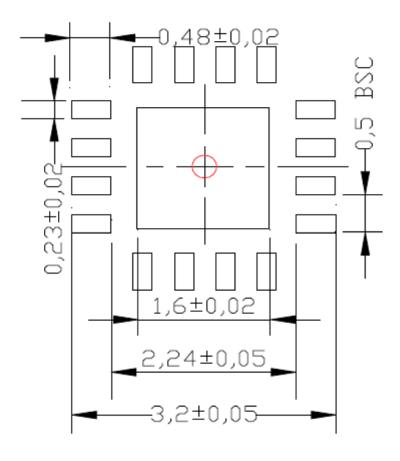
Red circle indicates Thermal Via. Size should be .300mm – .350mm in diameter and it should be connected to GND plane for maximum thermal performance. ALL UNITS ARE IN mm, TOLERANCE  $\pm 0.05$ , IF NOT NOTED LP # MLF33D-16LD-LP-1
