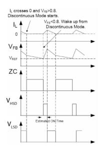
Figure 3b. MIC2103 Control Loop Timing (Discontinuous Mode)
