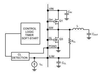
Figure 4. MIC2103/04 Current Limiting Circuit
