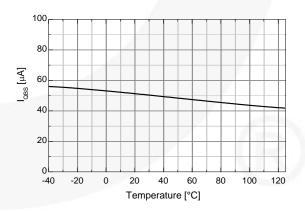
Figure 15. Quiescent V<sub>DD</sub> Supply Current vs. Temperature
