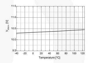
Figure 20.V<sub>DD</sub> UVLO- vs. Temperature
