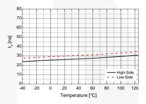
Figure 8. Turn-Off Fall Time vs. Temperature
