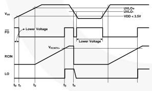
Figure 39. Waveforms for Under-Voltage Lockout
