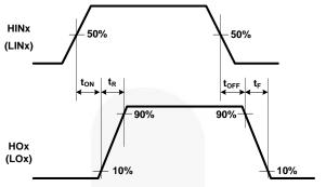
Figure 35. Switching Time Waveform Definitions
