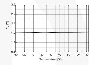
Figure 26.Logic LOW Input Voltage vs. Temperature
