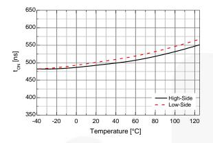
Figure 5. Turn-On Propagation Delay vs. Temperature
