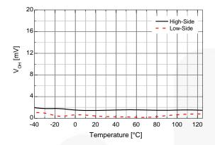
Figure 23.High-Level Output Voltage vs. Temperature
