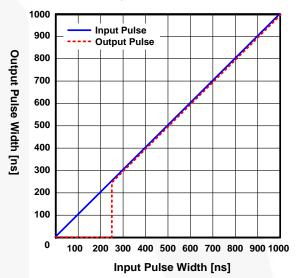
Figure 47.Input Filter Characteristic of Narrow ON
