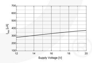
Figure 34. Operating V<sub>BS</sub> Supply Current vs. Supply Voltage
