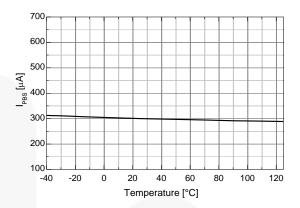
Figure 18. Operating V<sub>BS</sub> Supply Current vs. Temperature
