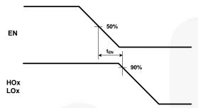
Figure 42. Output Enable Timing Waveform
