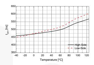
Figure 6. Turn-Off Propagation Delay vs. Temperature
