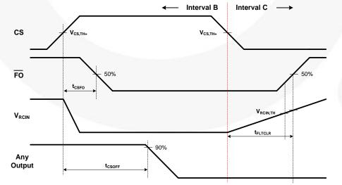
Figure 37. Detailed View of B and C Intervals During Over-Current Protection
