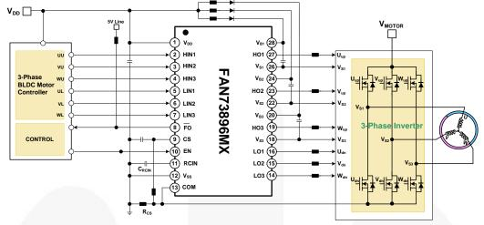
Figure 2. 3-Phase BLDC Motor Drive Application
