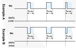
Figure 46. Noise Rejecting Input Filter Definition
