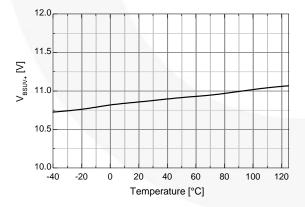
Figure 21.V<sub>BS</sub> UVLO+ vs. Temperature
