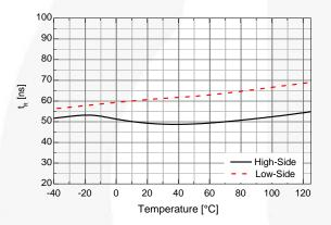
Figure 7. Turn-On Rise Time vs. Temperature
