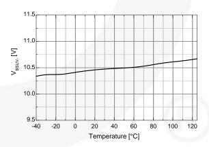
Figure 22.V<sub>BS</sub> UVLO- vs. Temperature
