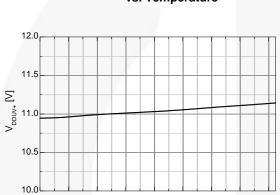
Figure 19.V<sub>DD</sub> UVLO+ vs. Temperature
