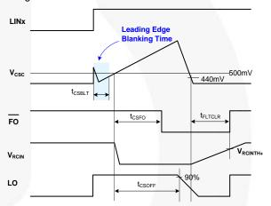
Figure 44.R<sub>CIN</sub> and Fault-Clear Waveform Definition
