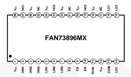
Figure 4. Pin Assignments
