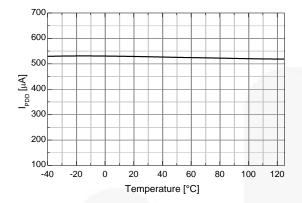
Figure 17. Operating V<sub>DD</sub> Supply Current vs. Temperature
