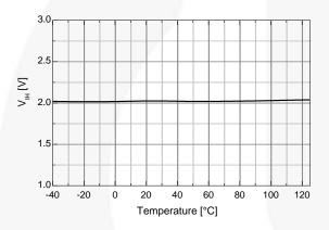
Figure 25.Logic HIGH Input Voltage vs. Temperature
