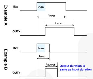
Figure 45. Input Noise Filter Definition
