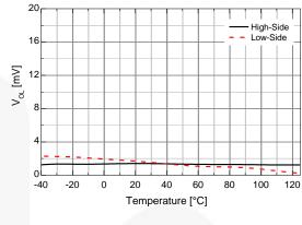
Figure 24.Low-Level Output Voltage vs. Temperature
