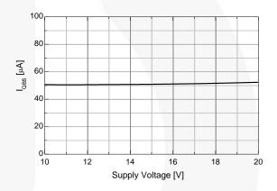
Figure 32. Quiescent V<sub>BS</sub> Supply Current vs. Supply Voltage
