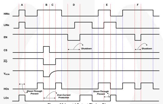
Figure 36.Input / Output Timing Diagram
