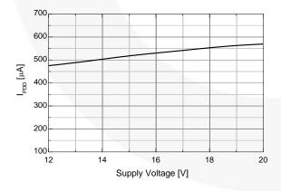
Figure 33. Operating  $V_{\text{DD}}$  Supply Current vs. Supply Voltage
