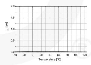
Figure 28. Logic Input LOW Bias Current vs. Temperature
