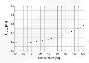
Figure 10. Fault-Clear Time vs. Temperature
