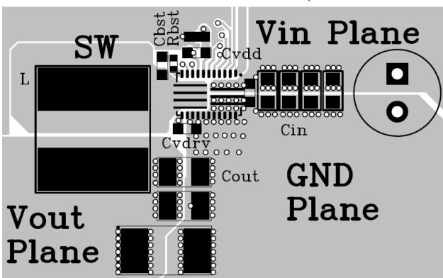
Figure 5: Sample PCB Layout
