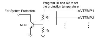
**Figure 4: System Thermal Protection**
