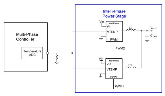
Figure 3: Multi-Phase Temperature Sense Utilization
