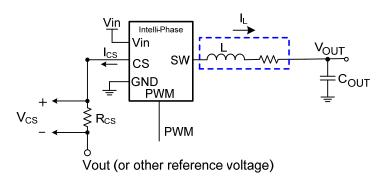
Figure 2: Replacing DCR Current Sense with Intelli-Phase's CS Output
