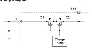
Figure 12: IN-to-SYS Pass-through Path
