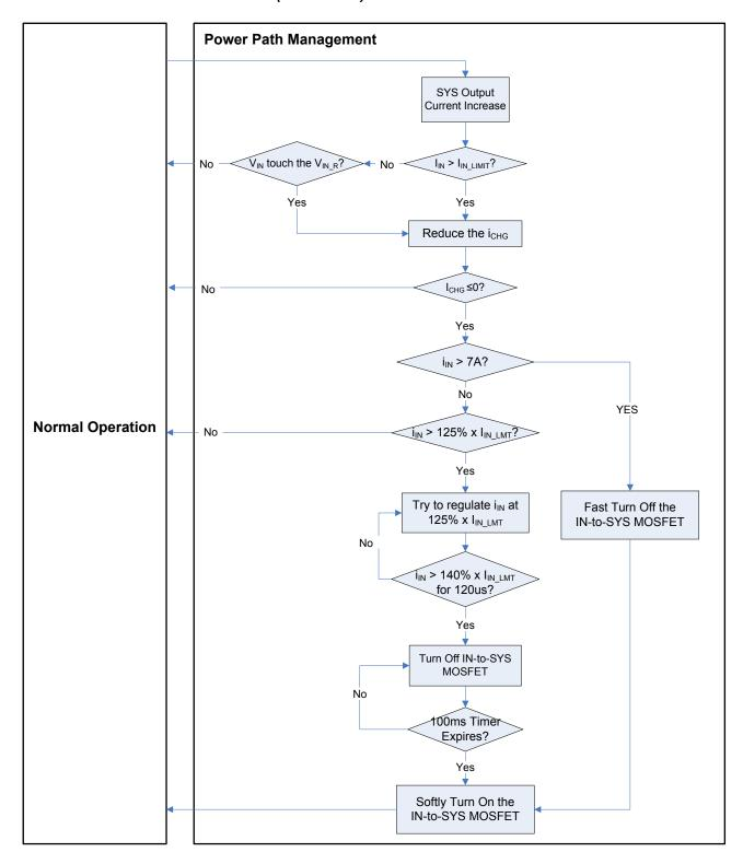
Figure 5: Power-path Management in Charge Mode
