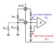
**Figure 14: NTC Function Block**
