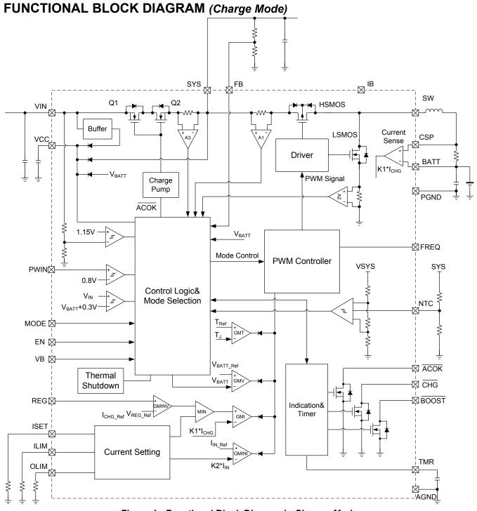
Figure 1: Functional Block Diagram in Charger Mode
