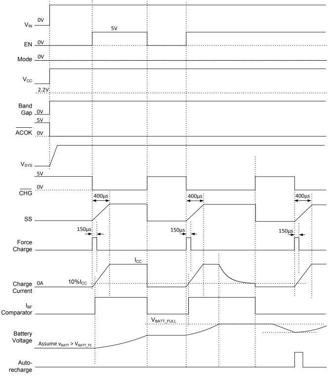
Figure 8: EN Start-up Time Flow in Charge Mode
