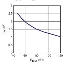
Programmable Input Current Limit, Charge Mode
