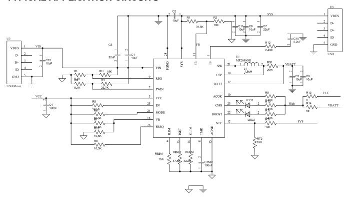
Figure 14: The Detailed Application Circuit of MP2636
