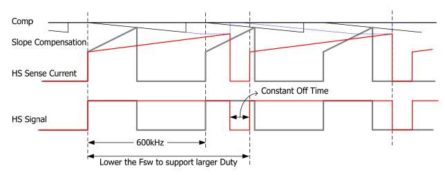
Figure 13: Constant-Off-Time Operation Profile
