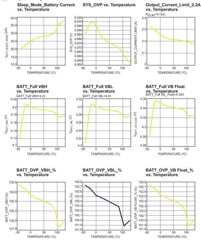
$V_{IN}$  = 5V (typ.),  $V_{BATT}$ =3.7V (typ.),  $C_{IN}$  =  $C_{BATT}$  =  $C_{SYS}$  = C2 = 22 $\mu$ F, L1 = 1.5 $\mu$ H, RS1 = 20m $\Omega$ , C4 = C<sub>TMR</sub> = 0.1μF, Battery Simulator, Unless Otherwise Noted.
