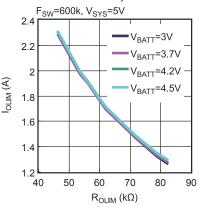
Programmable Output Current Limit vs. Battery
