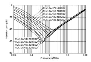
Common Mode Insertion Loss (Typ.)
