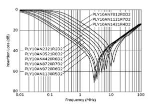
Differential Mode Insertion Loss (Typ.)
