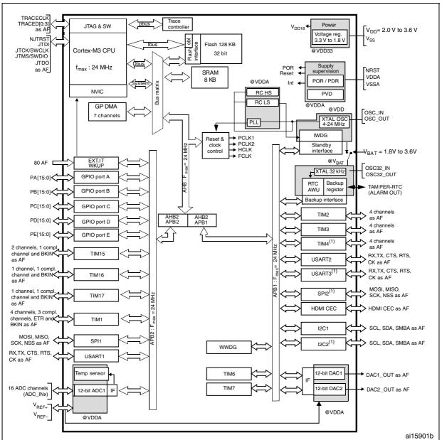
Figure 1. STM32F100xx value line block diagram
