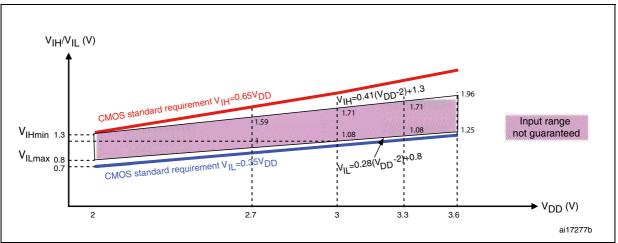
Figure 22. Standard I/O input characteristics - CMOS port
