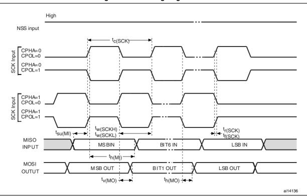
Figure 31. SPI timing diagram - master mode<sup>(1)</sup>
