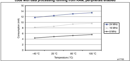
Figure 12. Maximum current consumption in Run mode versus frequency (at 3.6 V) - code with data processing running from RAM, peripherals enabled
