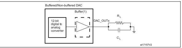
The DAC integrates an output buffer that can be used to reduce the output impedance and to drive external loads directly without the use of an external operational amplifier. The buffer can be bypassed by configuring the BOFFx bit in the DAC\_CR register.
