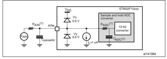
1. Refer to Table 42 for the values of  $R_{AIN}$ ,  $R_{ADC}$  and  $C_{ADC}$ .
