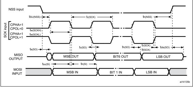
1. Measurement points are done at CMOS levels:  $0.3V_{\text{DD}}$  and  $0.7V_{\text{DD}}$
