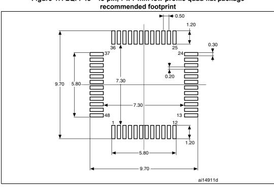
Figure 47. LQFP48 - 48-pin, 7 x 7 mm low-profile quad flat package
