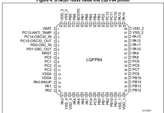
Figure 4. STM32F100xx value line LQFP64 pinout
