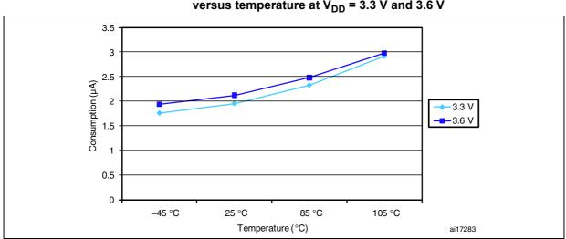
Figure 17. Typical current consumption in Standby mode versus temperature at  $V_{DD}$  = 3.3 V and 3.6 V
