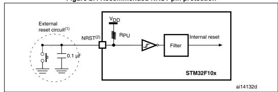
Figure 27. Recommended NRST pin protection
