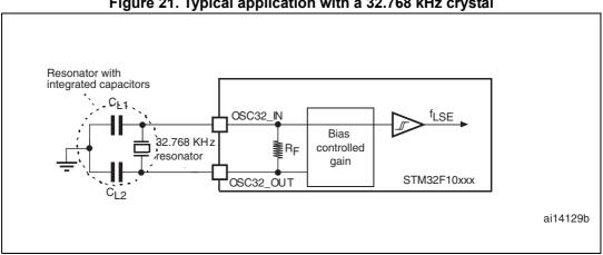
Figure 21. Typical application with a 32.768 kHz crystal
