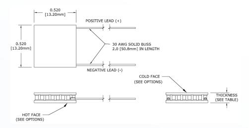
Ceramic Material 96% Alumina Ceramics Solder Construction: 232°C SnSb
