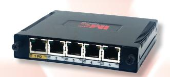
The (PoE) PD-Switch is a full-featured, 5-port 10/100Base-T MAC layer switch that extends the range of Ethernet networks, and increases port density, while being powered via IEEE 802.3af-compliant PoE through its "PD-port" (eliminating the need to run a separate power line for the device). Ethernet cabling usually runs only 100 meters; through the use of the PD-Switch, the outer range of an Ethernet network can be extended by an additional 100 meters.
