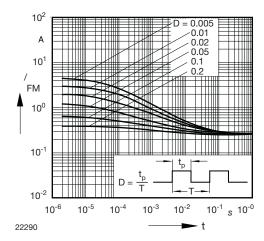
Fig. 2 - Peak forward current  $f_{fm} = f(t_p)$
