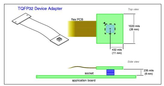
Figure 11: Device adapter critical dimensions
