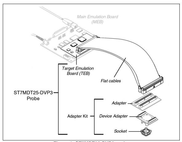
Figure 1: ST7MDT25-DVP3 probe
