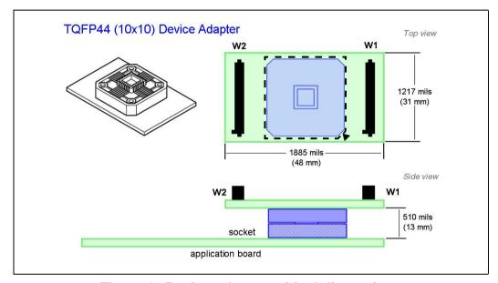
Figure 9: Device adapter critical dimensions
