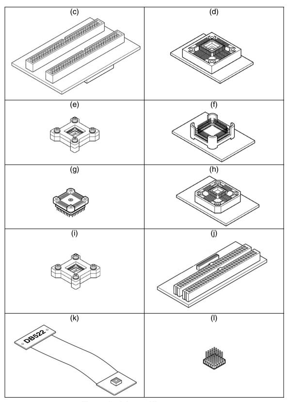
Figure 4: Adapter Kit components
