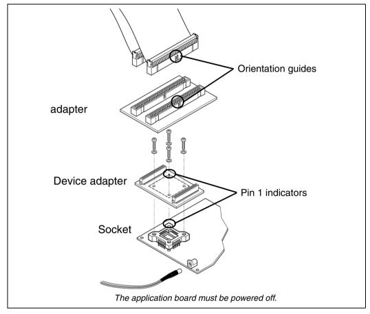
Figure 10: Connection for TQFP44 (10 x 10) package
