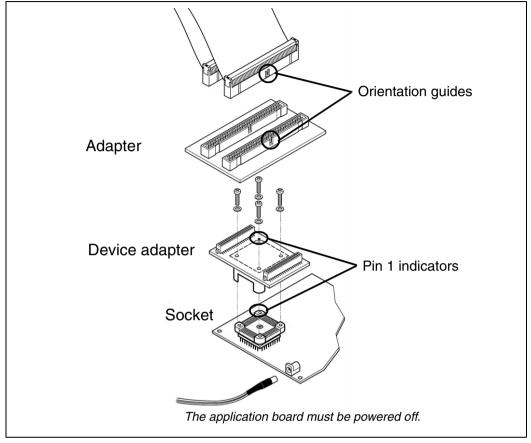
Figure 6: Connection for TQFP64 (14 x 14) package
