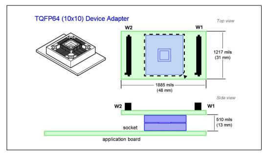
Figure 7: Device adapter critical dimensions
