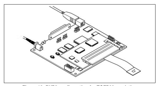
Figure 13: DVP3 configuration for TQFP32 emulation
