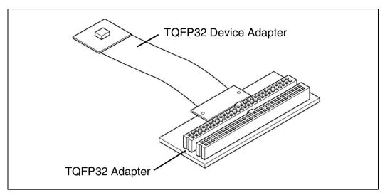
Figure 12: Flex PCB mounted on TEB adapter
