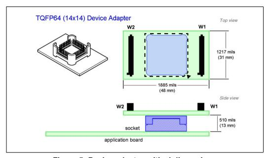
Figure 5: Device adapter critical dimensions
