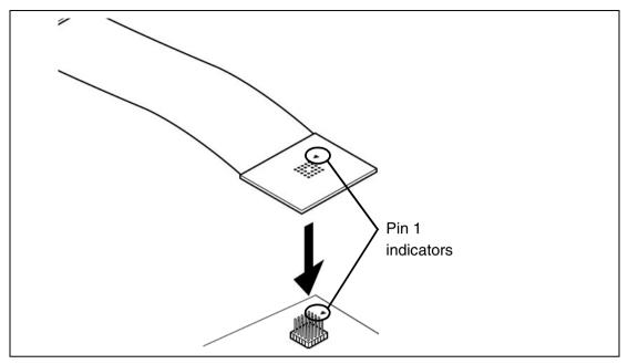
Figure 14: TQFP32 connector
