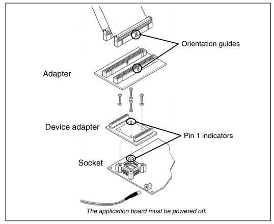
Figure 8: Connection for TQFP64 (10x10) package
